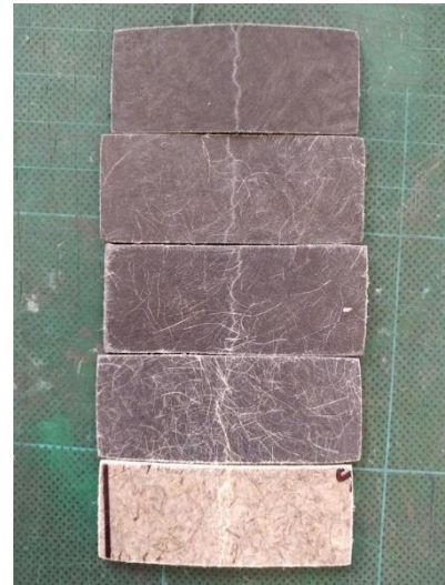
Figure 2: Recycled carbon fibre and flax fibre composite specimens after flexural tests show the effect of a higher flax content on the crack propagation.
