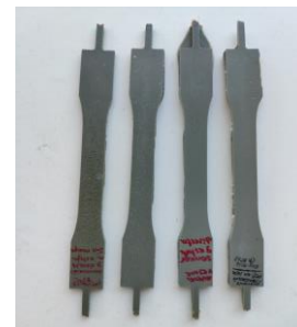
Figure 4: Tensile specimens based on SiC nanofilled bio-based epoxy resin from the European market.
