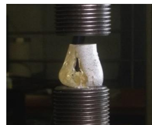
Figure 5: Compression test according to ASTM D695.
