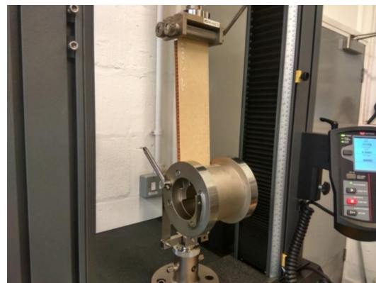
Figure 7: Set-up for peel test.
