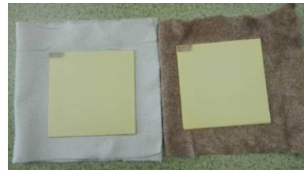
Figure 6: Plates manufactured with NF breather.
