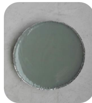
Figure 3 : Cured bio-based epoxy resin from European market nanofilled with silicon carbide nanoparticles.
