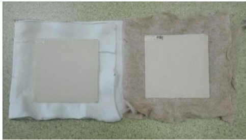
Figure 5 : Manufactured glass fabric panels (middle and high temperature).
