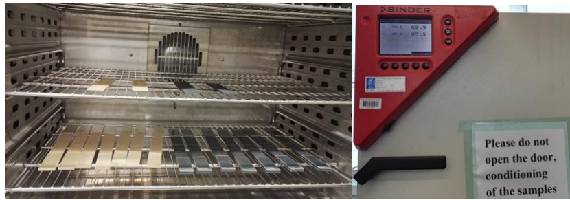
Figure 9: Hygrothermal ageing of composites in a conditioning chamber.
