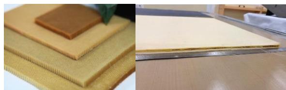
Figure 5: Sandwich panels made from green honeycomb and bio based prepreg.
