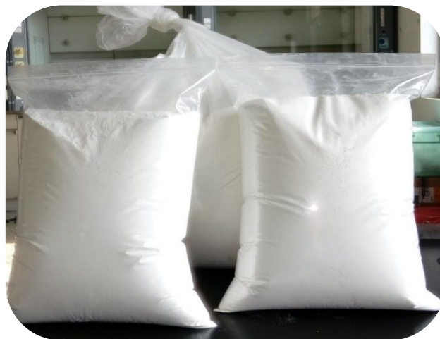
Figure 3: 60 kg batch of scaled-up rosin based curing agent by NIMTE.
