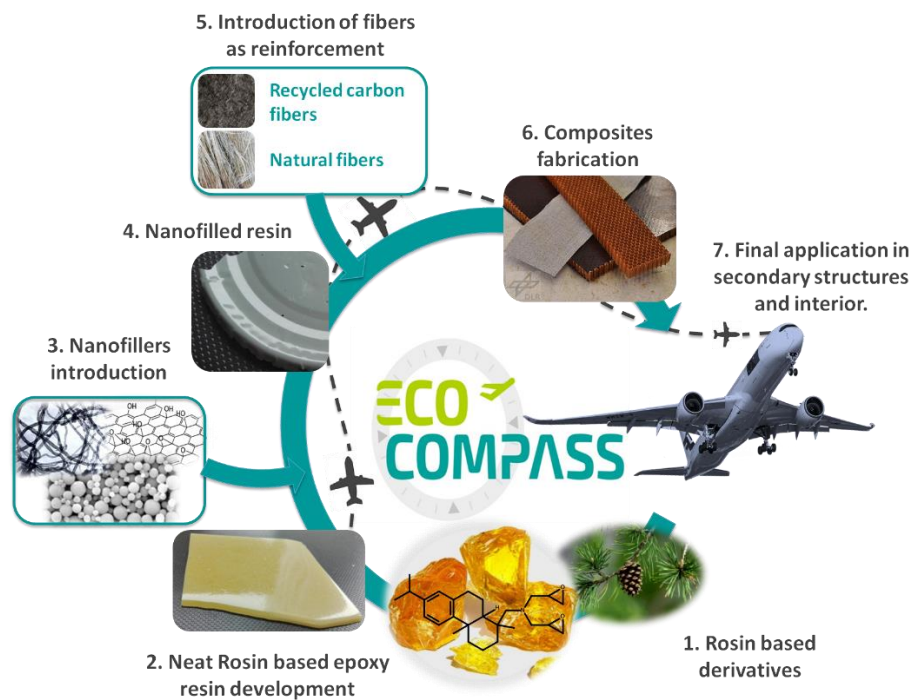
Figure 2: Rosin based resins manufacturing and application cycle.
