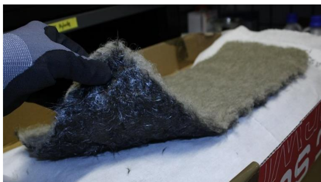
Figure 1: Hybrid gradient non-woven made of recycled carbon fibres and flax fibres.
