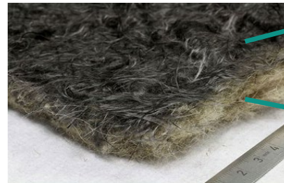
Recycled carbon and flax non-woven composite
